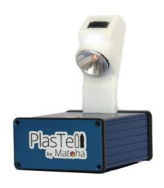
With PlasTell, you can make use of industrial standard infrared analysis techniques and cutting-edge machine learning algorithms, all in a tiny machine that is easy to operate and no scientific qualifications are required.
