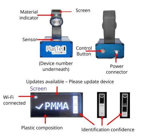
**Turn on**: plug in the power cable **Turn off:** unplug the power cable. **When starting**, the device will say "Calibrating". DO NOT place any samples onto the sensor until the device shows "Ready".
