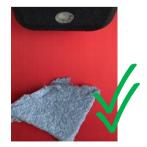
✓ DO cover the detector fully. If the sample is too small, place it on the right-hand side.
