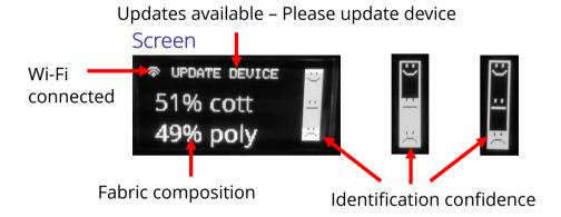
**Turn on**: plug in the power cable **Turn off:** unplug the power cable. **When starting**, the device will say "Calibrating". DO NOT place any samples onto the sensor until the device shows "Ready".
