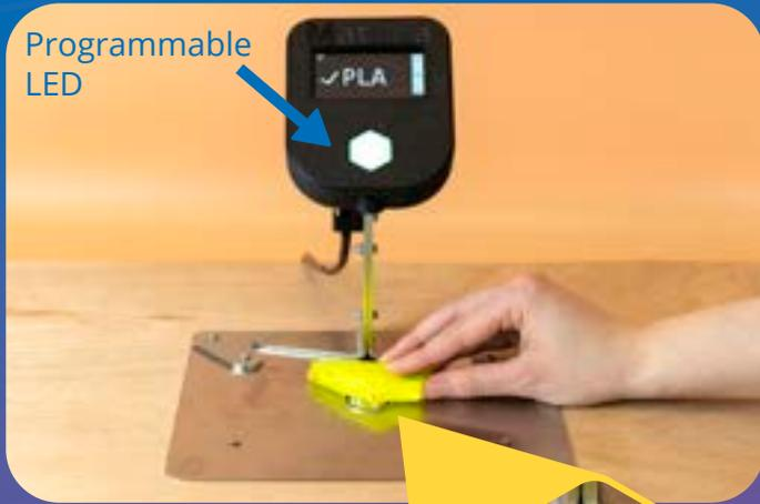
This allows you to mount the device on a wooden or metal bench and seamlessly add infrared plastics identification to your sorting process.
